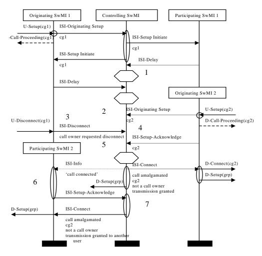
Figure E.11: Successful group call set-up: multiple calling parties an OSwMI transitions back into a PSwMI
