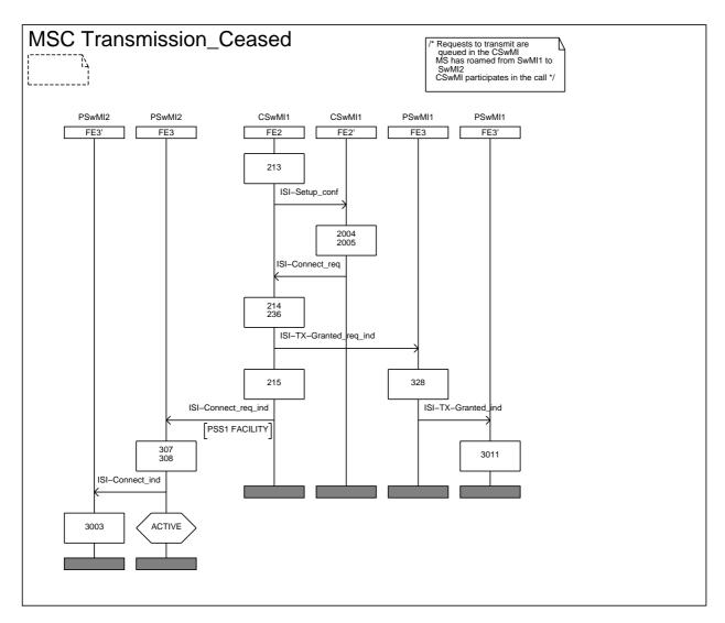
Figure 57: Information flow sequence -Permission to transmit following a cease transmission sequence (sheet 2 of 2) Figure 58 shows the information flow sequence for a request, to withdraw a non-granted transmission request, from a TETRA user in a participating SwMI.
