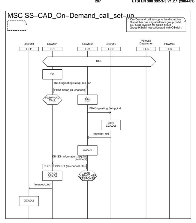
Figure B.9: Information flow sequence - On-demand call set-up (sheet 1 of 2)
