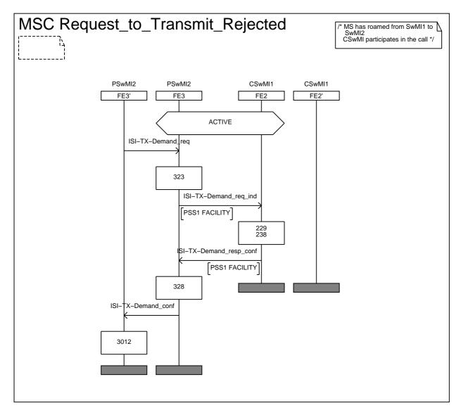
Figure 52: Information flow sequence - Request to transmit rejected
