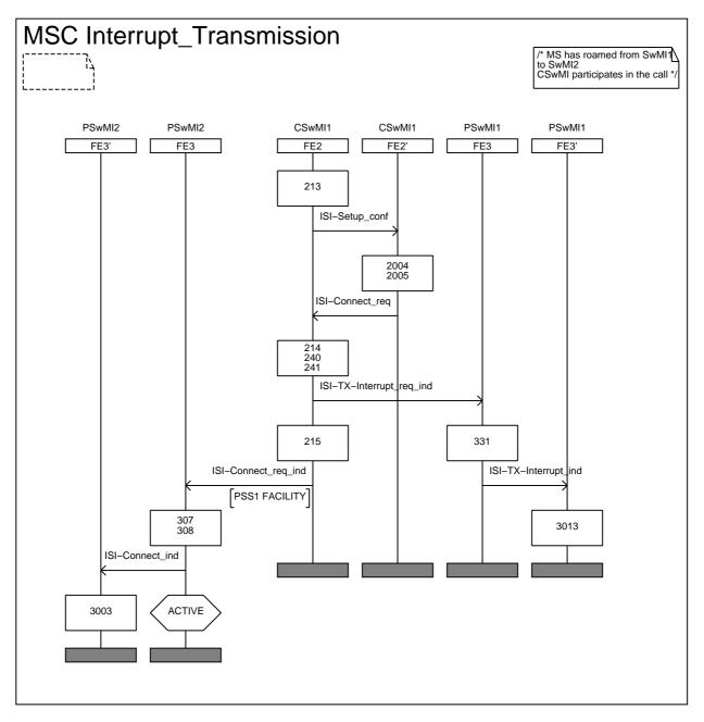
NOTE: If the parameter value, transmission grant in the ISI\_TX\_INTERRUPT PDU, is set to "transmission not granted", then an ISI\_RESOURCE PDU shall be sent to all participating SwMI(s) to check if resources are still available before an ISI\_TX\_GRANTED PDU is sent from the controlling SwMI. See figures 46 and 47 for an ISI\_RESOURCE PDU sequence.
