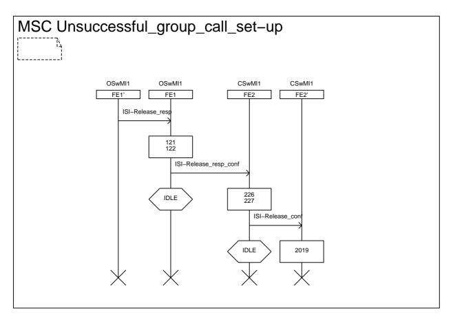
Figure 43: Information flow sequence - controlling SwMI rejects the call (sheet 2 of 2)
