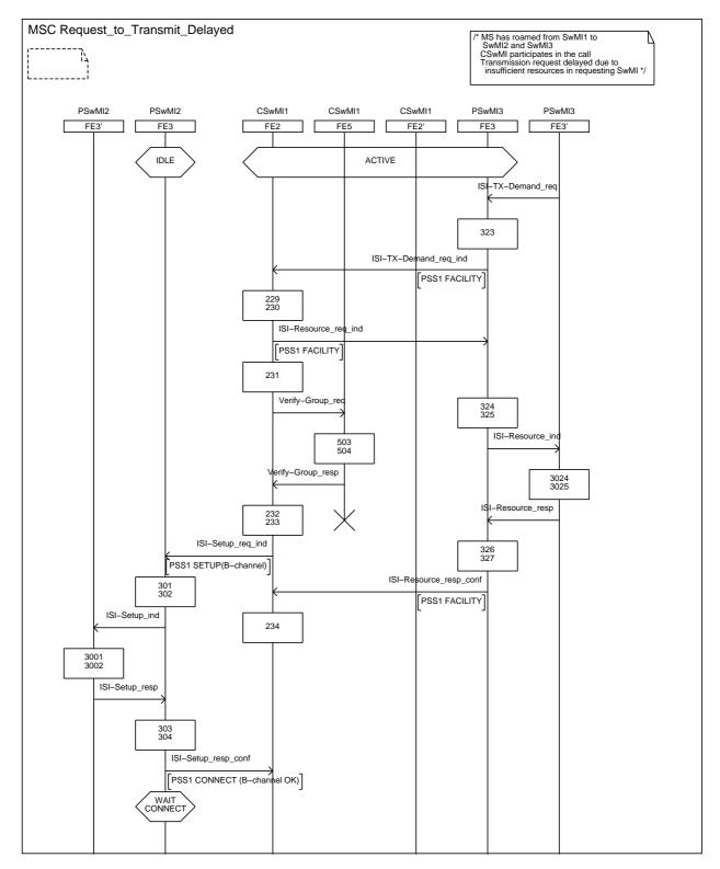
Figures 49 to 51 show the information flow sequence for a request to transmit from a TETRA user in a participating SwMI. The transmission request is delayed due to lack of resources.
